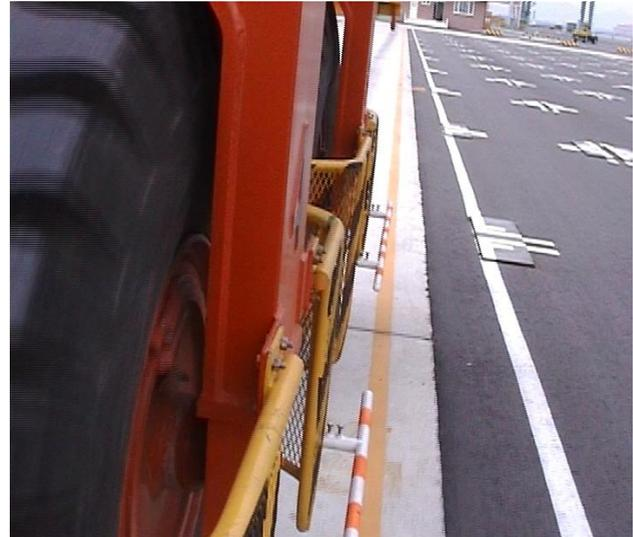
**Fig. 2 – Aligning the wheels of an RTGC to the line mark (yellow).**
