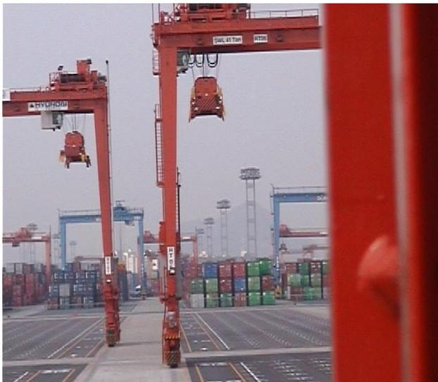
**Fig. 1 – Rubber-tired gantry cranes (RTGCs) tracking line marks.**
