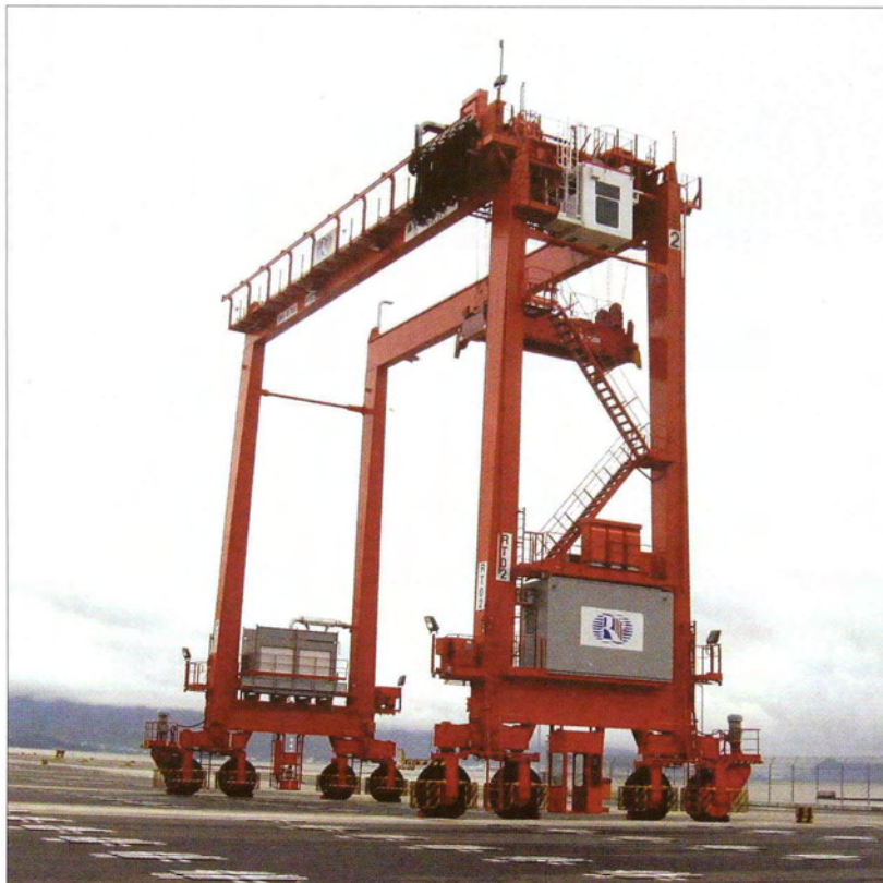
Figure 1, A rubber-tyre gantry crane; width 23m, height 21m
