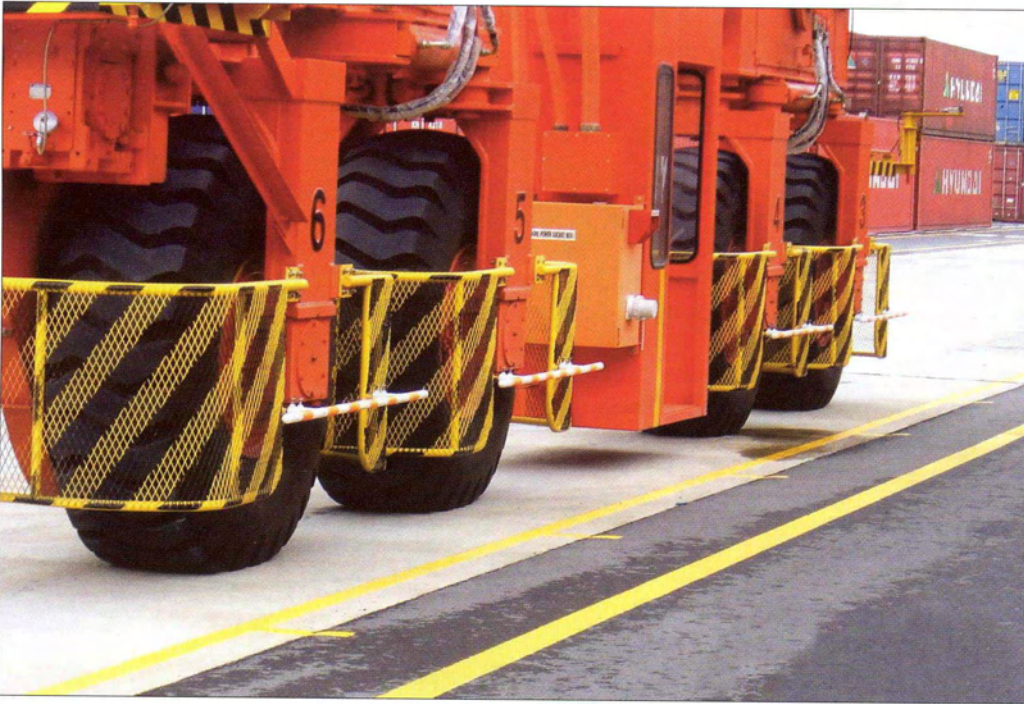
Figure 3, An RTGC's front and rear wheels moving along a concrete lane (corresponding to a virtual strip about 70 centimetres in width and 500 metres in length)
