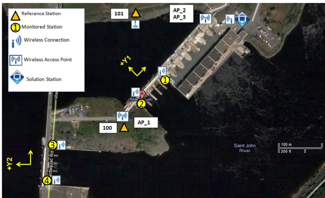
mmVu™ GNSS Monitoring Systems network with communications infrastructure at the Mactaquac dam.
