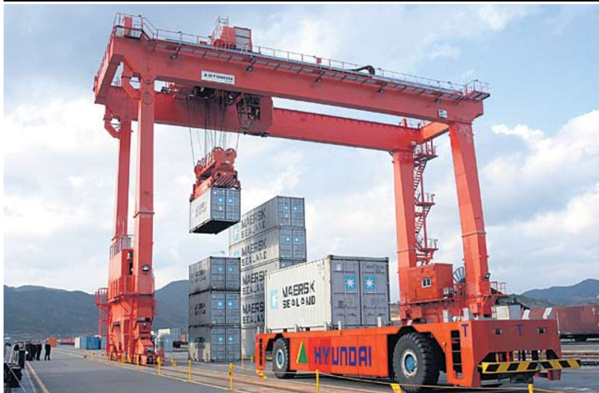
A gantry crane unloads a container in a demonstration of a programmable logic controller (PLC) system developed a few years ago by Dr. Don Kim and Dr. Jason Bond of the University of New Brunswick. Photo courtesy of Dr. Don Kim
